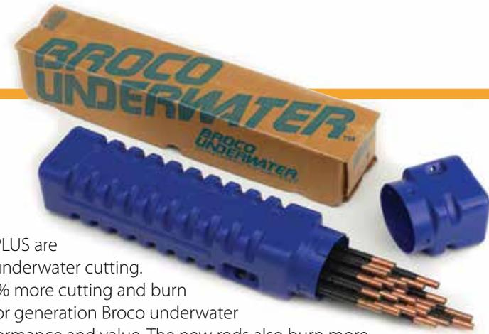
Burning in excess of 10,000°F at the tip, Broco underwater cutting rods cut and melt virtually any known material. Broco's patented rod design features alloy core wires retained by circular crimps, and a safety design to prevent burnback into the torch. Broco rods can be bent 90 degrees or more to access hard to reach places without restricting oxygen flow or causing insulation to split or flake off.
