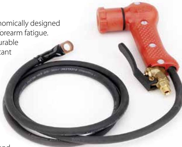
All connections are threaded for maintenance ease. The solid brass flash arrestor with internal filter protects the diver and torch without restricting oxygen flow. The large collet nut is knurled to assure the diver a solid grasp. Acme threads prevent binding from mud or other debris insuring quick, reliable rod insertion and retention. Interchangeable collets accommodate 3/8 inch, 5/16 inch or 1/4 inch diameter cutting rods.
